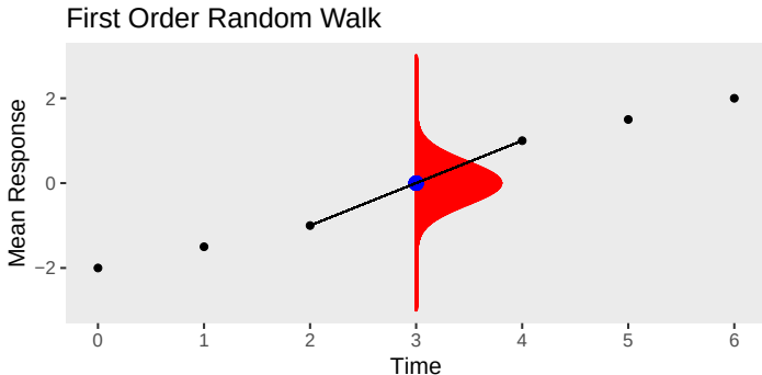
Figure 7: Illustration of the RW1 model for smoothing at time 3. The mean of the smoother is the average of the two adjacent points (and is highlighted as • ), and deviations from this mean are penalized via the normal distribution shown in red .
